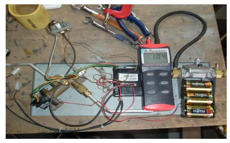
Next up is the actual measurement of the burner tube. I have attached a small fitting to the aeration port and sealed the ports with electrical tape. This should hopefully emulate the simulation setup.
