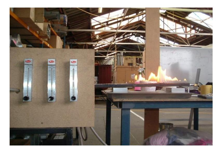
During the run of the flow measurement, I attach a manometer to the low pressure side of the regulator to make sure it has the proper inlet pressure: 1[kPa]
